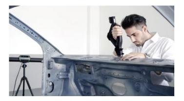
It can be paired with a tracking T-Probe (optional with different sizes) to probe inaccessible areas such as holes and hidden points. This contact measurement probe can ensure precise results with high single-point repeatability of 0.030 mm.
